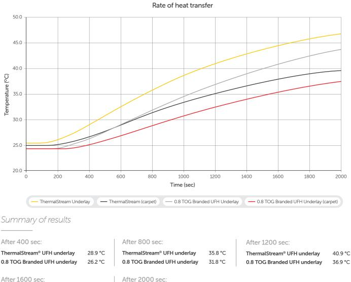
ISO 17025 Heat Transfer Results on a 200kw electric heat source Rate of heat transfer
